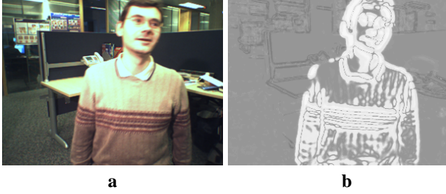
Figure 6. Testing the motion classifier. (a) A frame from the VK test sequence. (b) The corresponding motion likelihood map as output of a likelihood ratio test, see text for details. Bright pixels indicate motion (likelihood ratio R > 1 ) and dark ones stasis ( R < 1 ). Thanks to our joint motion likelihood strong stationary edges are assigned a lower (more negative, darker) value of R than stationary textureless areas.
