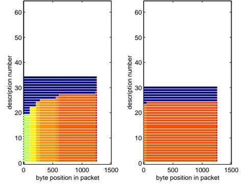
**Fig. 7.** Typical MDC base and enhancement layer packetizations using unequal erasure protection.
