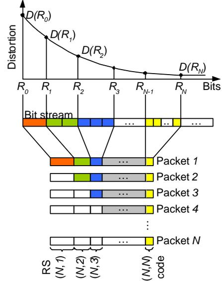
Fig. 2. Packetization for priority encoding transmission.
