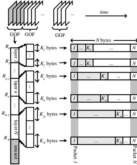
Fig. 1. Packetization for priority encoding transmission.
