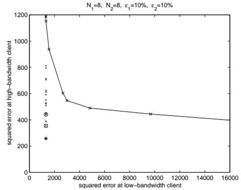
**Fig. 10.** Expected distortion of low-bandwidth client vs. expected distortion of high-bandwidth client for different layered MDC schemes, with 10% packet loss.  $N_1 = N_2 = 8$ .
