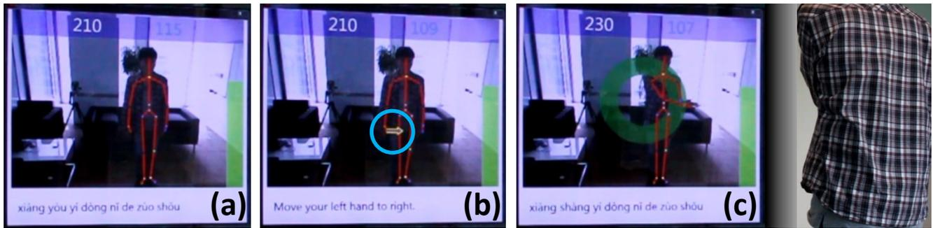
**Figure 2. Interactive Flow: (a) SpatialEase issues a command in Chinese; (b) if the user doesn't move or moves incorrectly, arrows are drawn on the video indicating the corresponding action; (c) the user performs the correct action and hear the next command.**
