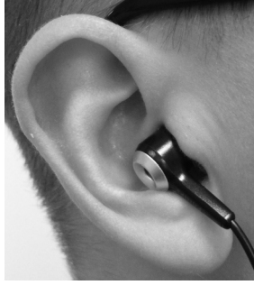
Figure 4.1: KAMARA headset . Microphones embedded into the headset record audio signals close to the ear canal entrances. Through the microphones a “pseudo-acoustic environment” is perceived [Härmä et al., 2003].
