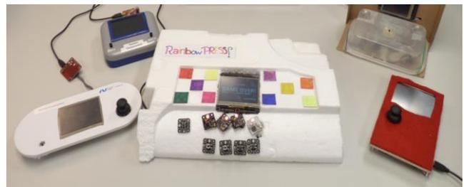
Figure 3. Prototype devices produced during a school pilot use a wide variety of materials to produce the required form-factors. These include (from left-to-right) printed cardboard, vacuum-formed plastic, expanded polystyrene, cardboard/plastic, and felt-over-cardboard.
