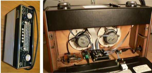
**Figure 9. Retro-fitting an existing product is a great way to build a robust prototype with a very specific form factor. Here we show a Roberts radio which has been ‘guttied’ and retro-fitted with Gadgeteer modules.**
