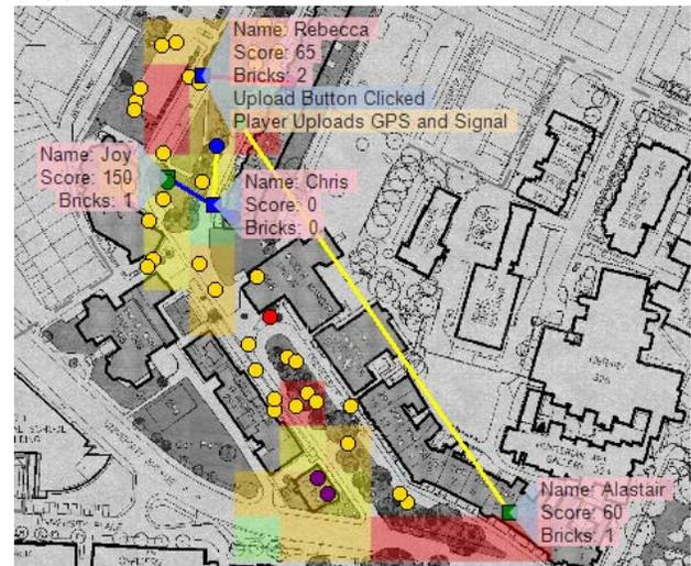
Screenshot of a visualisation of Bill – A mobile computing experience developed at Glasgow University. Yellow Lines indicate discrepancy between GPS position recorded on local device, and that available to the shared data space. Coloured overlay shows WiFi signal strength.
