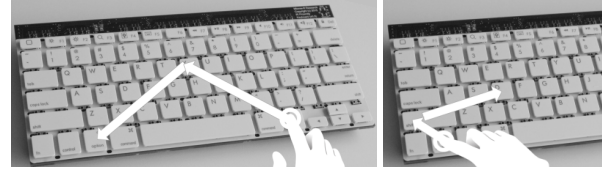
Figure 8. On-Keyboard shapes. Shape drawing to perform discrete commands. Physical keyboard as landmark may help as mnemonic aide in gesture memorization.
