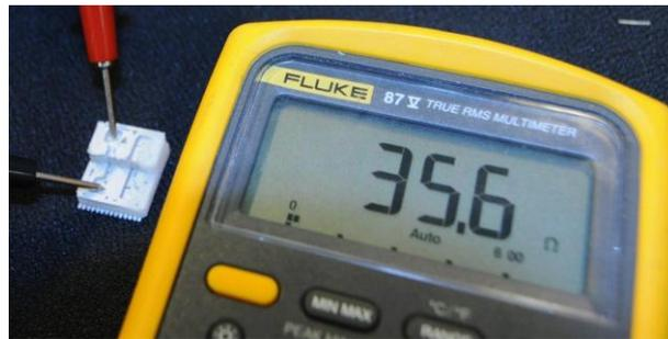
**figure 3.** a printed 3D dimensional trace
