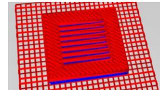
**figure 2.** masking test structure (ABS: blue, PLA: red)
