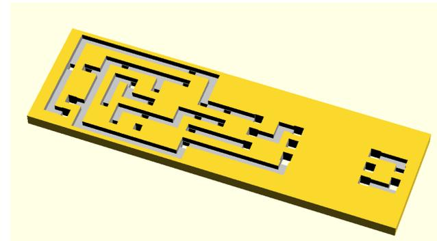
**figure 4.** printable PCB concept (ABS: yellow, Ag: silver)
