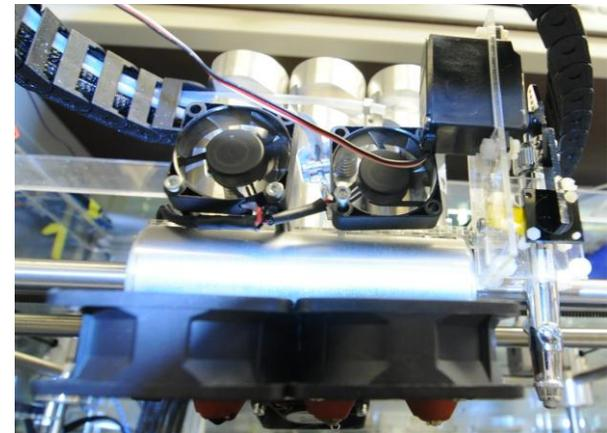
**figure 1.** extruder heads and airbrush
