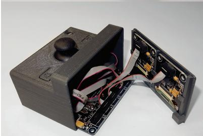
Gadgeteer modules [top] provide the hardware functions required for a DIY alarm clock. A CAD software package [screen shot, second from top] was used to design an enclosure, which was printed [second from bottom] using a 3-D printer. The modules were then fitted and connected [bottom].
