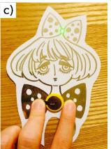
Figure 2: Example conductive ink circuits made in a workshop. Hand-drawn circuits typically combine a functional circuit with artistic elements, which often introduces electrical errors. When this happens the complexity of the conductive pattern makes it hard to analyze and repair the circuit.
