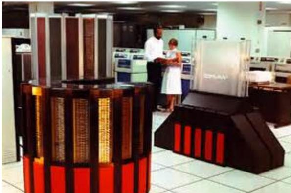
*Figure 9 Cray 2 with Fluorinert cooling*
