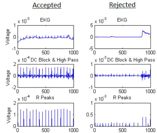
**Figure 2.** The rejected EKG signal (right) shows movement artifacts and variation in R peaks that is not seen in an accepted (left) signal.
