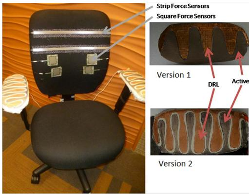
**Figure 1.** We employ conductive fabric on the chair's armrests to sense heart rate and pressure sensors on the back of the chair for sensing respiratory rate (left). Two iterations of our armrests (right).
