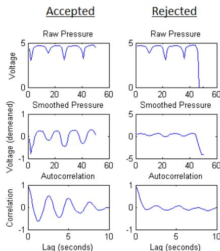
**Figure 3.** The accepted respiration signal(left) shows a much larger difference between the first valley and peak of the autocorrelation than the rejected signal (right).
