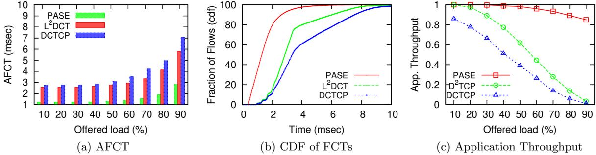
**Figure 9: (a) Comparison of PASE with L<sup>2</sup>DCT and DCTCP in terms of AFCTs under the (*left-right*) inter-rack scenario, (b) shows the CDF of FCTs at 70% load in case of (a), and (c) Deadline-constrained flows: Comparison of application throughput for PASE with D<sup>2</sup>TCP and DCTCP under the intra-rack scenario.**
