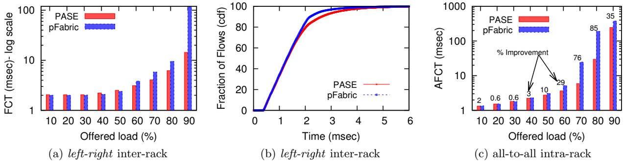
Figure 10: Comparison of PASE with pFabric under (a) 99<sup>th</sup> percentile FCT in the *left-right* inter-rack scenario, (b) CDF of FCTs under the *left-right* scenario at 70% load, and (c) all-to-all intra-rack scenario.
