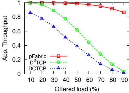
Figure 1: Comparison of two self-adjusting endpoint based protocols (D<sup>2</sup>TCP and DCTCP) with the state-of-the-art data center transport (pFabric).
