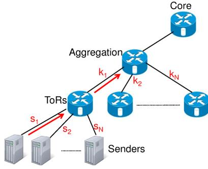
**Figure 6:** The *early pruning* optimization used by PASE for reducing the arbitration overhead. Note that  $s_i$  and  $k_i$  represent flows that are mapped to the highest priority queue at the senders and the ToR arbitrators, respectively.
