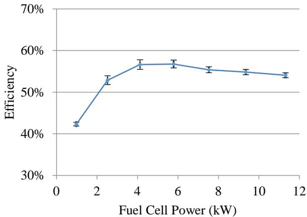
**Figure 3. The efficiency curve of the 12kW in-rack PEMFC system. Error bars in the data indicate  $\pm$  one standard deviation from 5 different measurements.**
