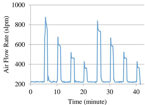
**Figure 8. The cathode air flow rate during the series of step load changes.**
