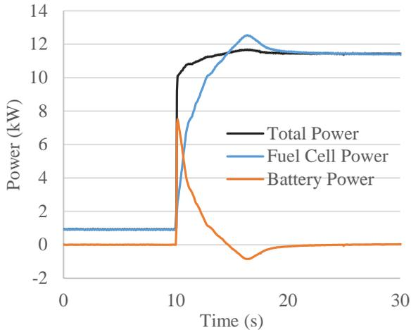
**Figure 5. The power profiles of the PEMFC system, the battery and the total output power, the external load changes from 0kW to 9.0kW at t=10s.**
