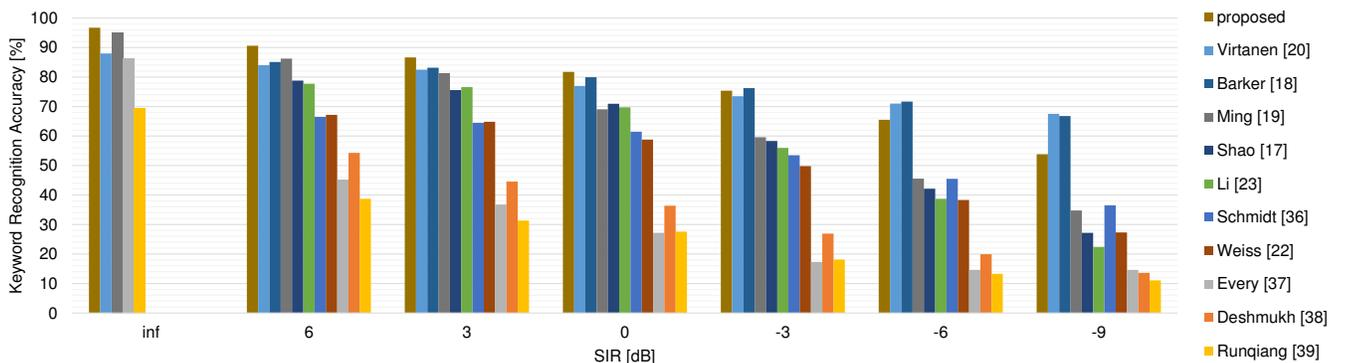
**Fig. 4.** Performance comparison of different solutions for co-channel speech recognition on the SSC task. Bars show average percent keyword recognition accuracy across DG and SG test conditions at different SIR levels. All compared solutions use HTK in their ASR experiments.
