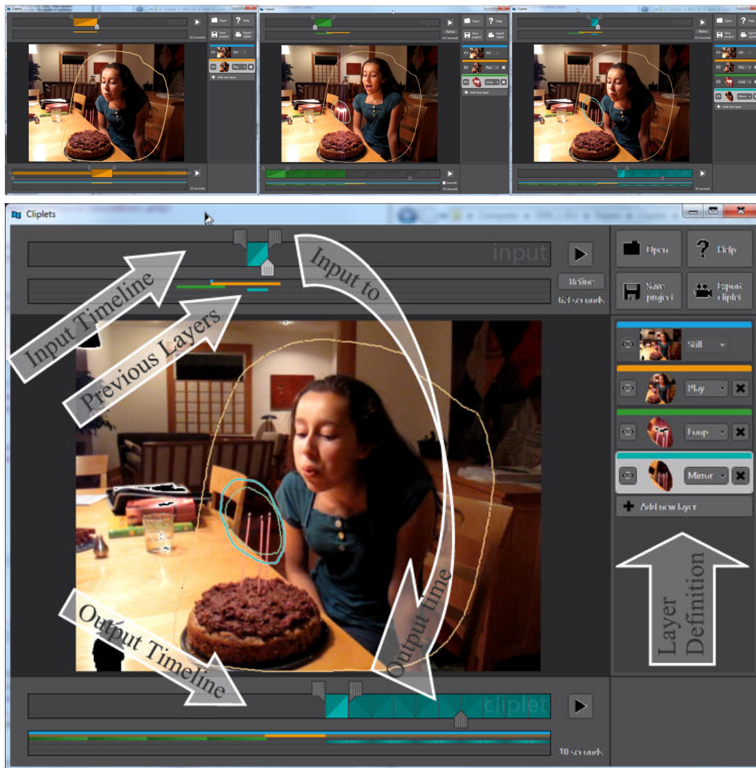
Figure 3: Interactive system for creating cliplets. The main area is used to indicate the spatial boundaries of layers and show the input video and resulting cliplet. The input and output timings for each layer are defined on the top and bottom timelines, respectively. The top three panels depict the process of defining a play layers, followed by a loop, and a mirror layer in sequence. [Click on the bottom image to play a video show the entire session of construction this Clippet.]
