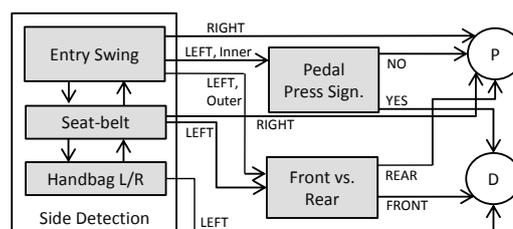
Figure 1: Using sensor data to determine if the mobile user is a driver or a passenger. P = passenger, and D = driver.
