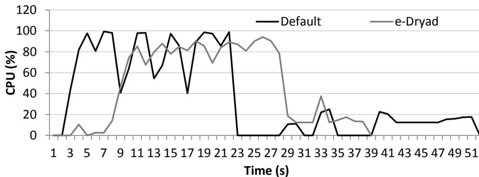
Figure 5: Resource utilization with and without e-Dryad.
