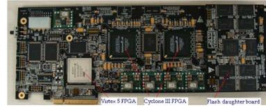
Figure 1: The customized board with 36 Flash chips
