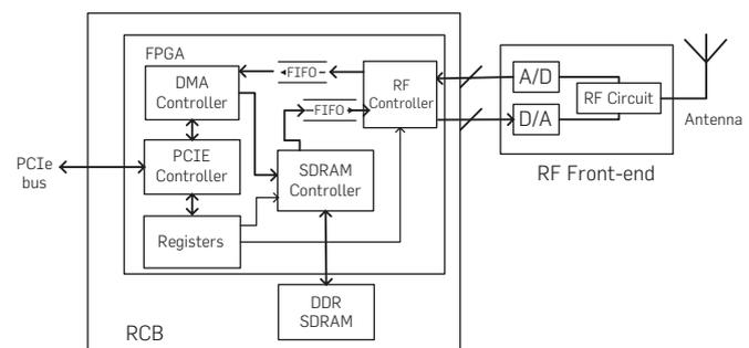
in a DMA burst (128B). When transmitting, the large RCB memory enables Sora software to first write the generated samples onto the RCB, and then trigger transmission with another command to the RCB. This functionality provides flexibility to the Sora software for precalculating and storing several waveforms before actually transmitting them, while allowing precise control of the timing of the waveform transmission.
