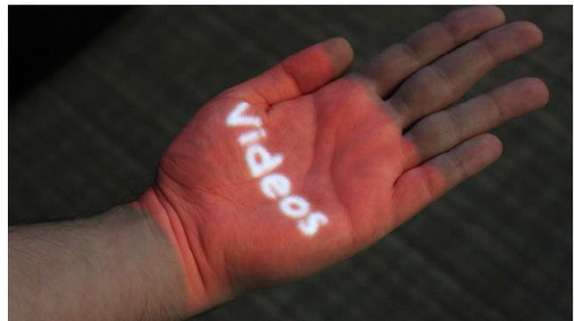
Figure 10: By aligning the projectors and the cameras, we can correctly project virtual content registered with the real world. In this case, we project a menu option directly onto the user's hand.
