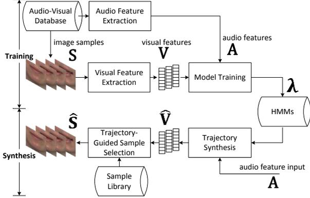
Fig. 1. Synthesis framework with trajectory-guided sample selection.
