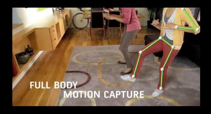
Body skeleton tracking using a depth camera
