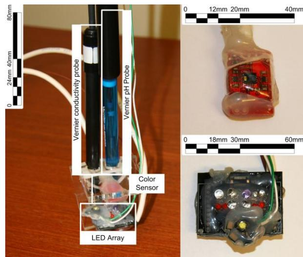
Figure 5. (left) Prototype sensor package. The sensor is submerged inside a drink along with the pH and conductivity sensors to record a fingerprint of the liquids response to various illumination sources. (right – top) Avago ADJD-S71 color sensor (right – bottom) LED color array
