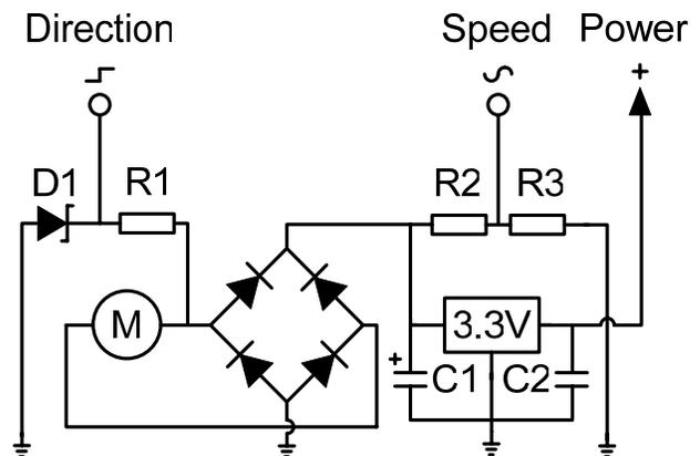
**Figure 3. A simple circuit that enables human-powered rotary input devices.**
