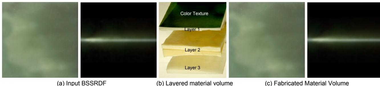
**Figure 1:** Our system automatically generates a layered material volume for approximating a custom BSSRDF. (a) The appearance of a real material sample under diffuse lighting and a beam light. (b) A collection of layers generated by our system for assembling the output volume. (c) The appearance of the fabricated material volume under the same diffuse lighting and beam light.
