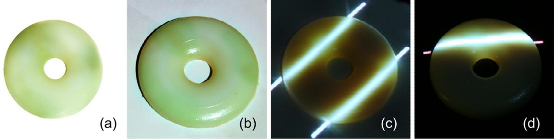
**Figure 11:** Fabricated round plate with designed jade-like subsurface scattering. (a) The input BSSRDF rendered with diffuse light. (b) Photograph of fabricated round plate under diffuse light. (c)(d) Appearances of the fabricated round plate captured under different lightings. The object size is 82mm × 82mm × 9mm
