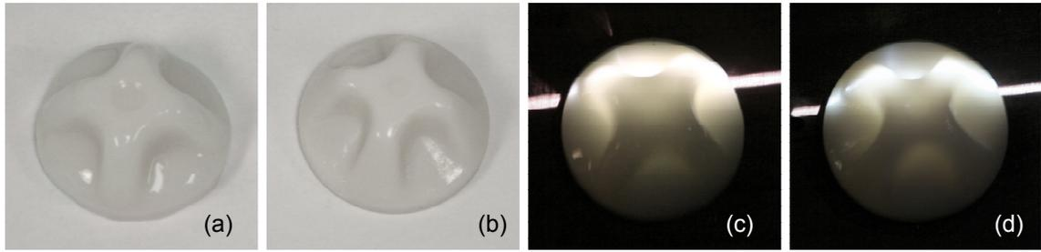
**Figure 10:** Fabricated jello. (a) A real piece of jello, the homogeneous BSSRDF of which is used as input to our system (b) A fabricated piece of jello generated by 3D printer. (c) Photograph of the real piece of jello under line lighting. (d) Photograph of the piece of fabricated jello under the same line lighting. The real jello and the fabricated one have the same size of 50mm × 50mm × 27mm
