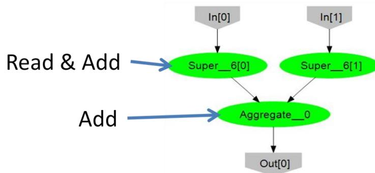
Figure 9: Aggregation of associative function is done using multiple machines.
