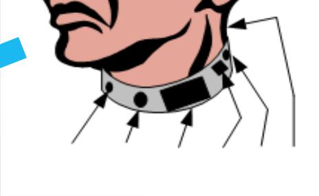
Sleep apnea neck cuff with oximeter, accelerometer, microphone, & gsr sensors
