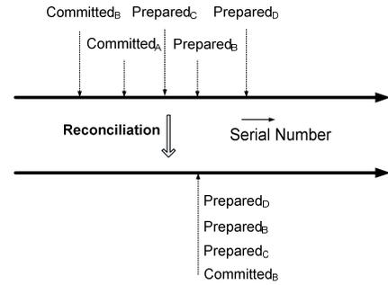
**Figure 1: Reconciliation: An Example.**  $A$  was the primary in the old configuration. In the new configuration, an old secondary  $B$  is promoted to be the new primary with  $A$  removed from the configuration. The first line shows the state of the prepared lists and the committed lists of the replicas based on the highest serial numbers on the lists. The second line shows the corresponding state after reconciliation.
