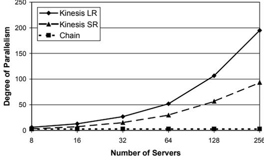
Figure 9: Kinesis(7, 3) vs. Chain(3): Degree of Parallelism with Varying Numbers of Servers.
