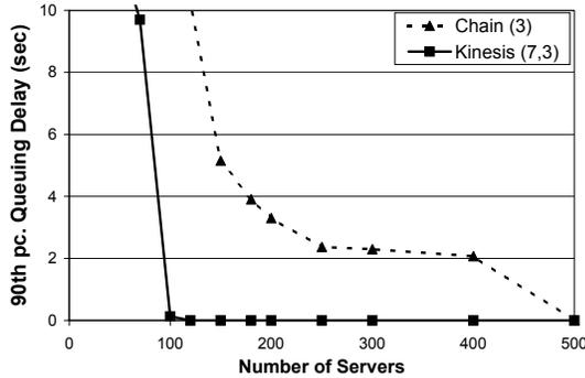
Figure 5:  $Kinesis(7, 3)$  vs.  $Chain(3)$ : 90th percentile queuing delay for read requests on MSN Video trace, as the number of servers is varied with average read request rate fixed at 2.9 GB per second.
