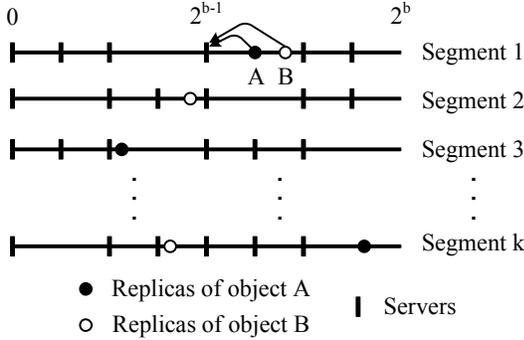
Figure 1: Kinesis Data Placement Model: Kinesis divides the servers into  $k$  segments, employs independent hash functions to map an object to a unique server in each segment, and replicates the object in  $r$  servers chosen from the  $k$  mapped servers based on resource availability.
