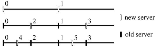
Figure 2: Key-Space Distribution in Linear Hashing
