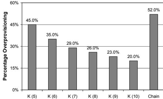
Figure 3:  $\text{Kinesis}(k, 3)$  vs.  $\text{Chain}(3)$ : Over-Provisioning Percentage:  $\text{K}(k)$  corresponds to  $\text{Kinesis}(k, 3)$  and  $\text{Chain}$  to  $\text{Chain}(3)$ . Kinesis requires substantially less additional storage capacity than Chain to handle the same workload.
