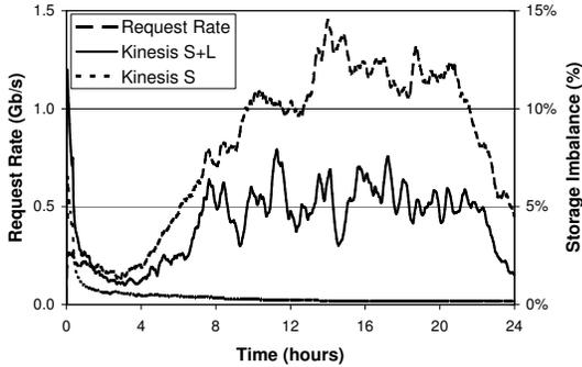
Figure 8: Storage Imbalance vs. Time: Kinesis S+L compensates for temporary decreases in storage balance when client activity is low.
