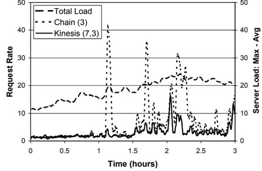
Figure 10: Network-Load Imbalance vs. Time: Kinesis(7, 3) balances network load significantly better than Chain(3) during high request loads.
