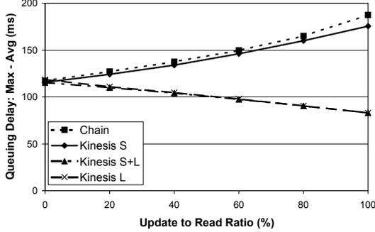
Figure 7: Network-Load Imbalance vs. Update-to-Read Ratio: Kinesis S+L provides comparable load balance to Kinesis L despite the influence of storage consumption while balancing load.
