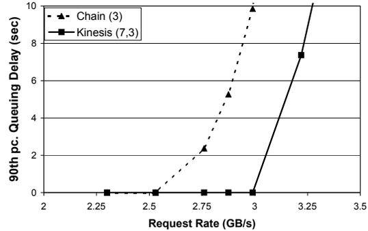
Figure 6:  $Kinesis(7, 3)$  vs.  $Chain(3)$ : 90th percentile queuing delay for read requests on MSN Video trace, as average read request rate is varied with a number of servers fixed at 128.
