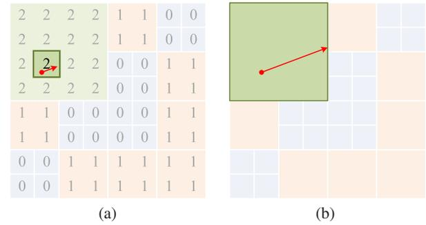
**Figure 5:** Adaptive photon marching using an octree. (a) The photon's position is used to determine the level of the surrounding leaf node of the octree. (b) The step size  $\Delta s_{\text{octree}}$  is calculated to advance the photon to the boundary of the octree node.
