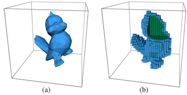
**Figure 3:** (a) A triangle-mesh surface representation of an object. (b) The same object after conversion to volumetric data by our voxelization method (partially cut away to show the interior).
