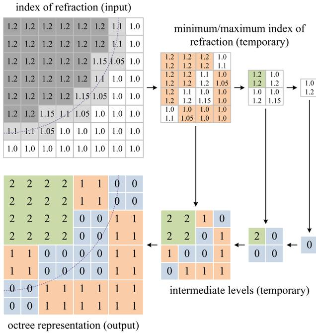
**Figure 4:** Octree construction algorithm, simplified to 2D. We first build a pyramid containing minimum and maximum refractive index values. We then analyze the pyramid from the coarsest level to the finest, writing the current level number into the octree representation whenever the range of refractive index values is within the input tolerance  $\varepsilon = 0.05$ .
