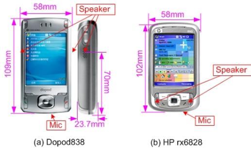
Figure 1. Two COTS mobile devices used in the evaluation of BeepBeep ranging system.
