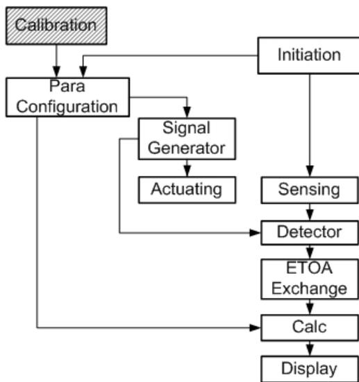
Figure 2. Procedure flow in BeepBeep ranging system.
