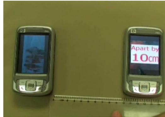
Figure 3. One snapshot of BeepBeep ranging experiment using HP iPAQ rw6828.
