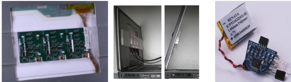
**Fig. 2.** Our proof-of-concept prototype uses three sensor PCBs mounted in a portrait orientation behind the LCD (left). The resulting assembly is not much thicker than the LCD panel itself; the acrylic mounting strip used for expedience in the prototype is the thickest part (centre). Our prototype embedded IR receiver supports data communication from the display (right).
