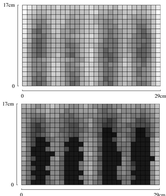
**Figure 7. The best-case scenario (top) and the worst case (bottom) for a case of bottled water moving past the reader**
