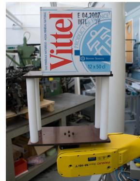
**Figure 1. The product holder, shown with a product (a case of bottled water) ready for testing**
