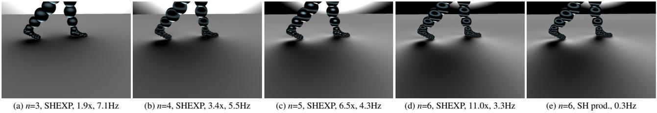
Figure 8: SH order comparison. Factors like “1.9x” in (a) are the increase in speed of the SHEXP method over the SH product method of the same order. Timings were done on a CPU-only rendering using  $200 \times 200$  shaded vertices on the ground plane and  $n_S=60$  shadowing spheres (no hierarchy).
