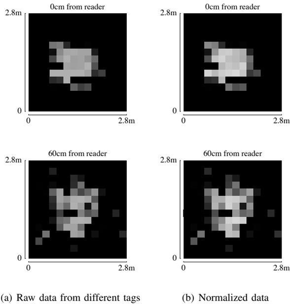
Fig. 9. The effect of normalization on the data. Slices taken parallel to the face of the reader at increasing distances.
