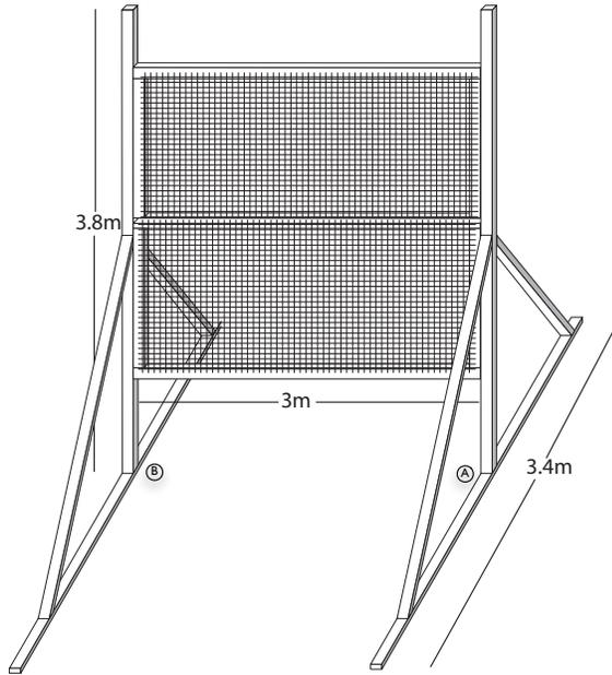
Fig. 2. The frame which supported the grid of tags. It was constructed entirely of wood, with plastic mesh stretched over the frames for rigidity and a sheet of thin plastic taped on top of that to accurately attach the tags to.
