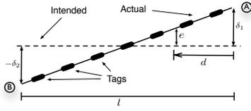
Fig. 1. The placement error due to an array, a plan view of Fig. 2.
