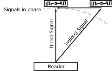
Fig. 3. Phase differences caused by reflections. When the reflected and direct signals meet they are out of phase, and can either add to or subtract from each other, depending on the phase difference.
