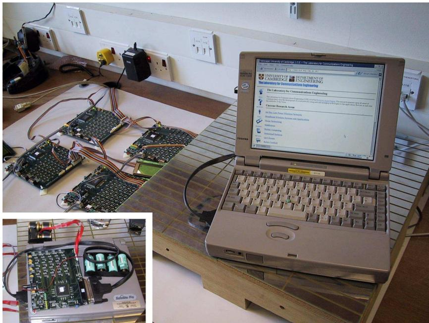
Figure 2.9: Photograph of LVDS Object on Prototype Surface
