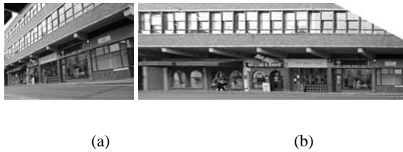
Figure 11: Plane rectification via partial internal parameters. (a) Original image. (b) Rectification where the relative scaling of vertical and horizontal directions assumes a natural camera with the principal point at the centre of the image. The focal length is computed from the single orthogonal vanishing point pair. Measurement of the aspect ratio of a window indicates a difference of 3.7% between true and computed values. Note that the two parallel planes, the upper building facade and the lower shopfront, are both correctly rectified, but scene planes not parallel to these two are distorted by the rectification homography. This distortion is visible on the area of overhang of the upper facade.
