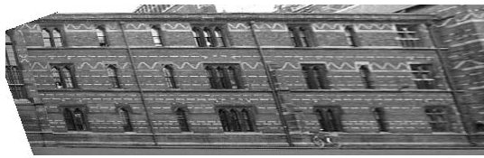
Figure 5: The affine rectified image. Notice that parallelism is restored, but angles and ratios of lengths are still incorrect.
