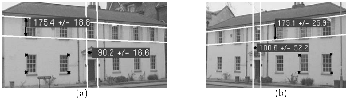
Figure 5.6: Crystallography labs Oxford - The actual height of all the windows is 174 cm, the door width is 100 cm.
