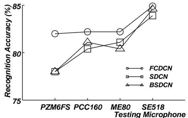
**Figure 2:** Comparison of recognition accuracy for SPHINX on the alphanumeric task using four microphones and the BSDCN and FCDCN algorithms. The system was trained using speech from the CLSTLK microphone.
