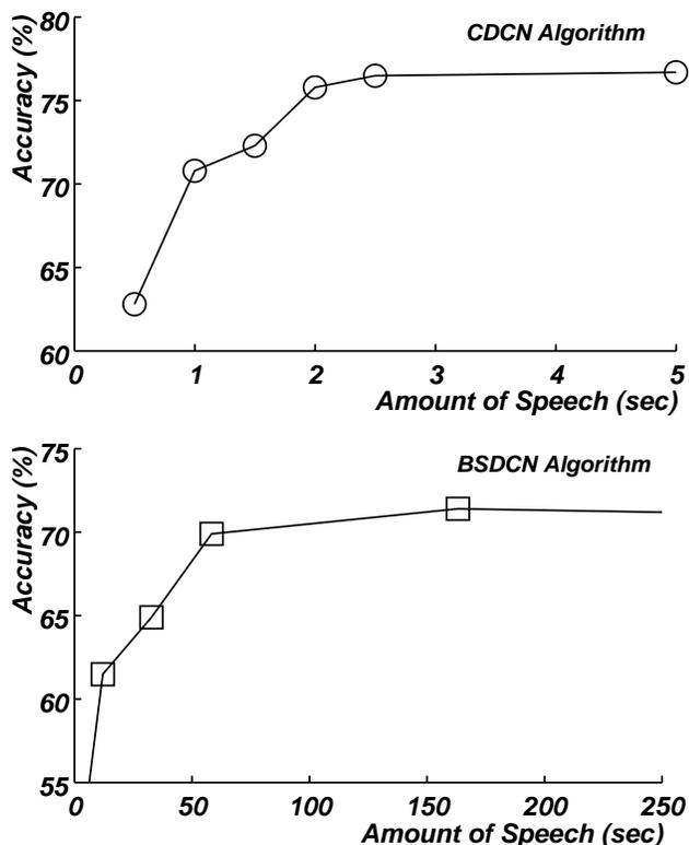
**Figure 3:** Dependence of recognition accuracy of the CDCN and BSDCN algorithms on the amount of speech in the testing environment available for adaptation. The system was trained using the CLSTLK microphone and tested using the PZM6FS.
