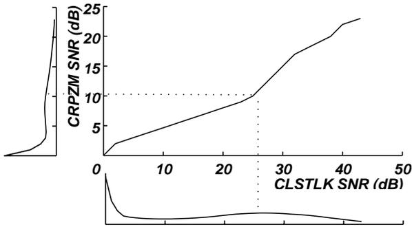
**Figure 1:** Nonlinear mapping of SNRs for the CLSTLK and PZM6FS microphones based on histograms of SNR values. The unlabeled graphs along the horizontal and vertical axes indicate the relative likelihood of observing various SNRs for the two microphones. The central panel indicates the warping path that best matches the two functions.
