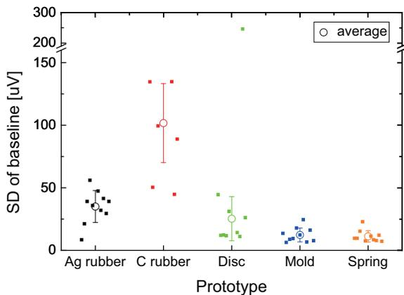
Figure 7. SD median represents stability of the baseline. Right two prototypes show excellent performance. Though “Ag rubber” is inferior compared with the two, the difference is not critical.
