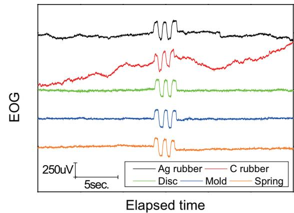
Figure 5. Observed EOG in a part of Figure 4. Eye movements are clearly found in all prototypes; some prototypes offer excellent stability.
