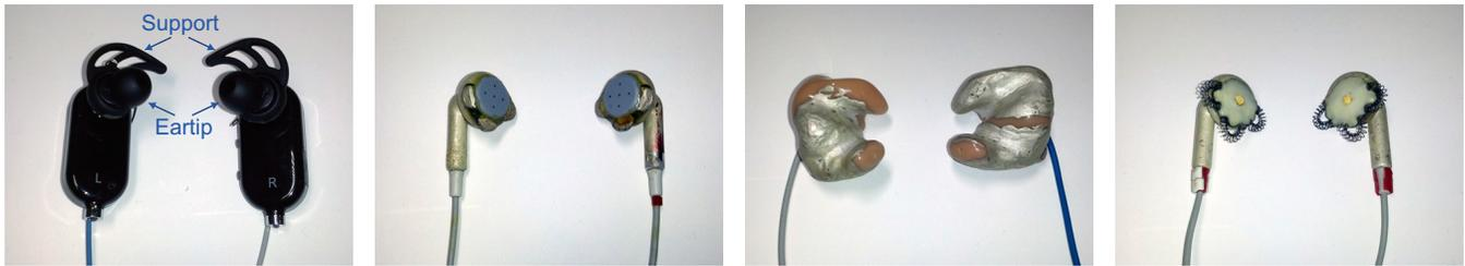
Figure 1. Prototypes tested. Starting from the left, “Rubber”, “Disc”, “Mold” and “Spring”. Each pair of earphones has at least 3 independent electrodes.
