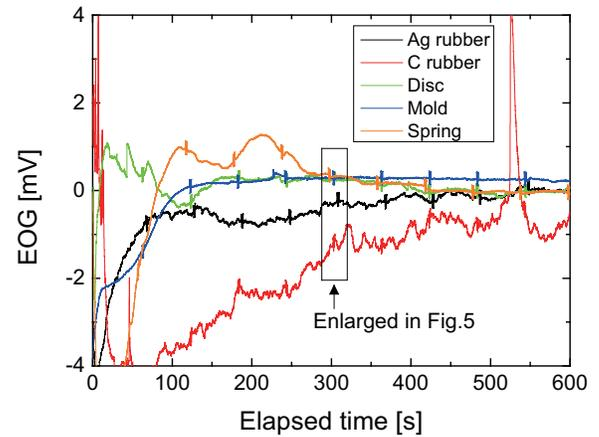
Figure 4. An example of EOG according to Figure 3. Eye movements every one minute are found as small and quick swings. Baseline stability differs with the prototype.
