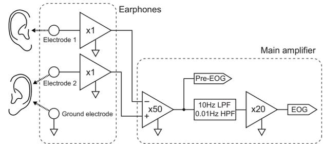
Figure 2. Simplified schematic for EOG measurement. Electrodes 1 and 2 are placed on different sides (right and left) and ground electrode can be placed on either side.
