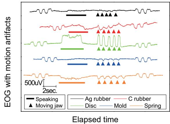
Figure 8. Measured EOG during motions. While “Disc” introduces quite large motion artifact, “Ag rubber” and “Mold” have high tolerance.
