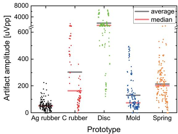
Figure 10. Artifact amplitude introduced by moving jaw. Artifacts with “Ag rubber” are smaller than eye movement in many cases.
