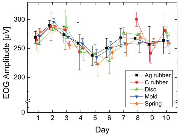
Figure 6. Measured EOG amplitude. Though the values change with day slightly, all prototypes capture the eye movements to the same level.
