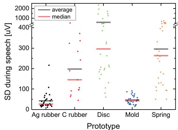
Figure 9. SD during speech section. Artifacts with “Ag rubber” and “Mold” are smaller than others
