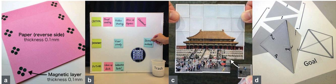
**Figure 1. FluxPaper and its applications: (a) Basic structure of FluxPaper, (b) Automated To-do list by whiteboard and electromagnet header behind the board, (c) Creating picture puzzle using 25 pieces of self-aligned paper, (d) Tetrahedron model using self-aligned paper.**
