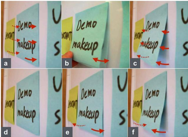
**Figure 13. Paper Expressions:** (a) attraction to avoid user to remove the paper, (b) vibration to notify the task is not finished or failure, (c) curl-up to get user’s attention, (d, e, f) waving makes noise to notify.
