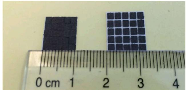
Figure 5. Samples of FluxPaper with non-slit and slit design.
