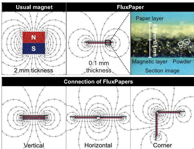
Figure 2. Illustration of FluxPaper and magnetic pole.
