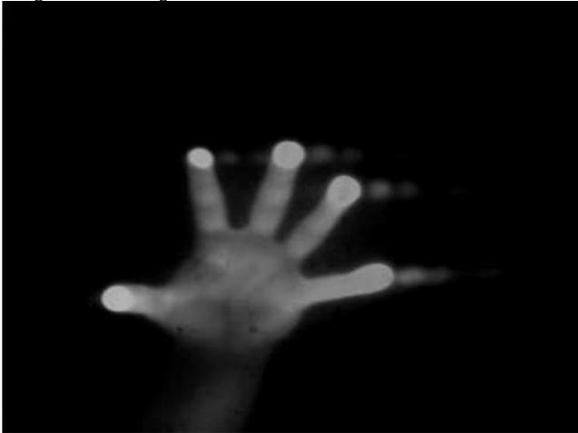
Fig. 23: A hand touching the screen, imaging at infra-red wavelengths with a wedge camera through an LCD (uses a leaky front light diffuser)
