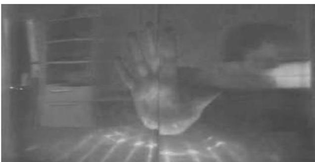
Fig. 25: Detection at visible wavelengths through a transparent OLED using a pair of Wedge cameras. The center vertical line is the stitch-line between the two wedges
