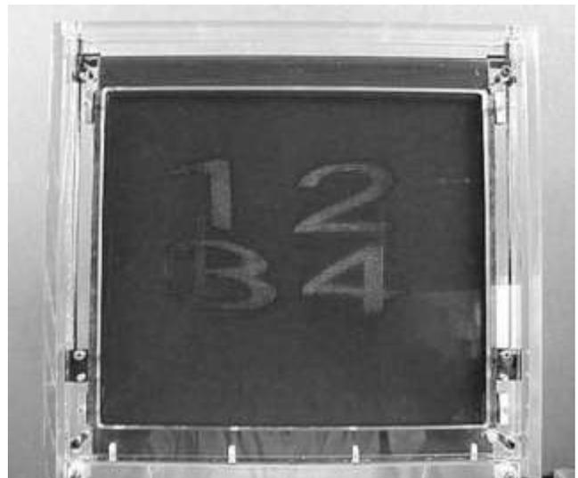
Figure 12: Photograph of image projected through a wedge of borosilicate glass tapering linearly from 1.5 mm to 0.5 mm over a distance of 200 mm
