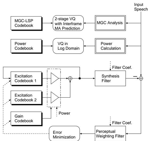
Figure 1: Structure of wideband MGC-CELP coding.
