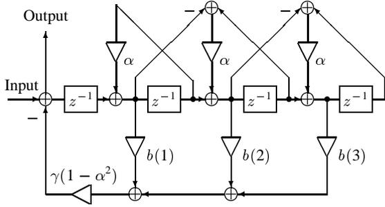
Figure 2: Structure of  $1/C_1(\tilde{z})$  for  $M = 3$ .
