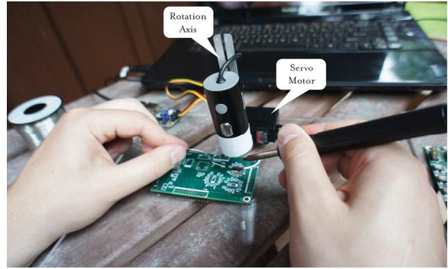
Figure 2. The hardware components in Scopemate.
