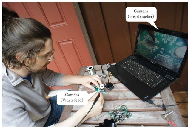
**Figure 1.** Our tracking inspection microscope setup.
