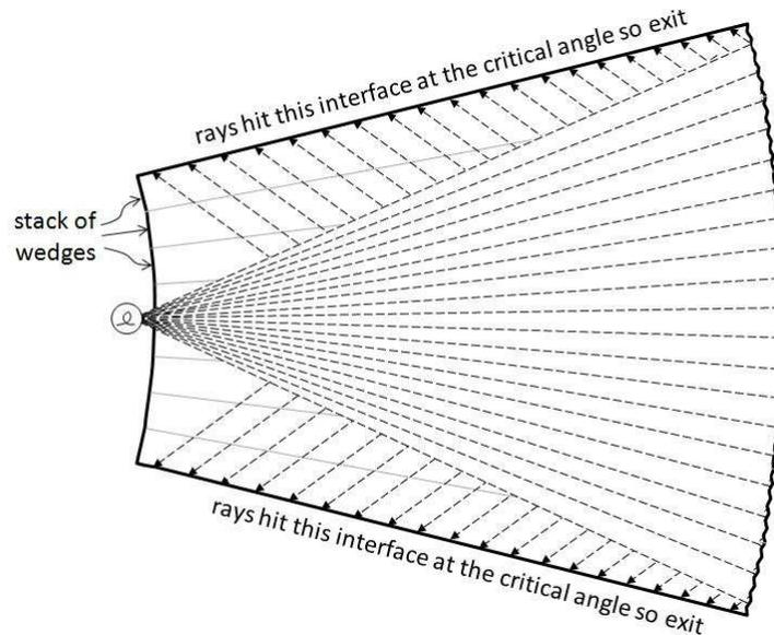
Fig. 3. Rays travel as if through a stack of wedges. The curvature of the thick end collimates the rays and the facets slew the direction of collimation so that rays illuminate the whole of the surface as they reach the critical angle.
