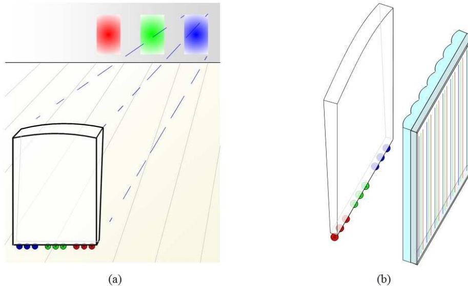
Fig. 4. The wedge collimates rays from each source in a direction determined by its position (a). Hence a cylindrical image of the sources is formed by each lenticule on the adjacent column of pixels in the liquid crystal display (b).
