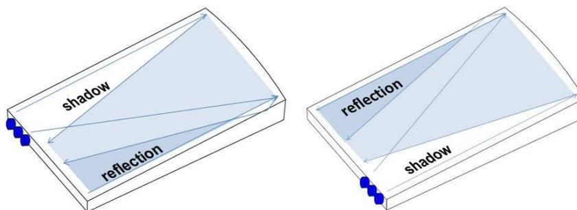
Fig. 5. Rays from LED's either side of the center will leave a shadow.
