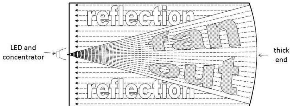
Fig. 1. Plan view: rays fan out to the thick end where they are reflected in parallel.
