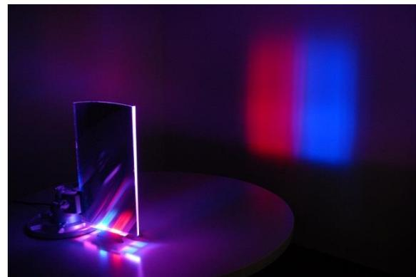
*Figure 2: Projection onto screen 2 metres from a wedge backlight with 30 mm separation between red and blue sources at input*
