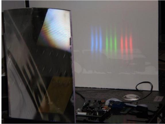
*Figure 3: Projection from a wedge backlight via a 450mm focal length Fresnel lens onto a 570 mm distant screen*
