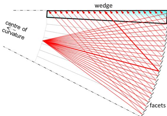
*Figure 1: The thick end is curved and faceted so as to concentrate ray paths to a point at the input*
