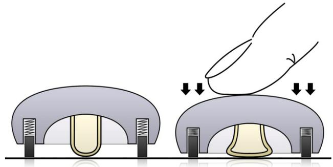
Figure 1. A simple pressure sensitive button increases contact area with increasing downward force.
