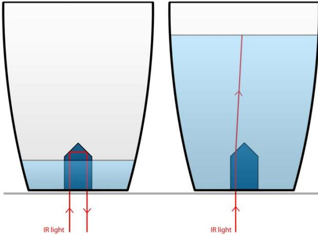
Figure 4. A SurfaceWare glass uses a prism-like structure to reflect light when it is not submerged.
