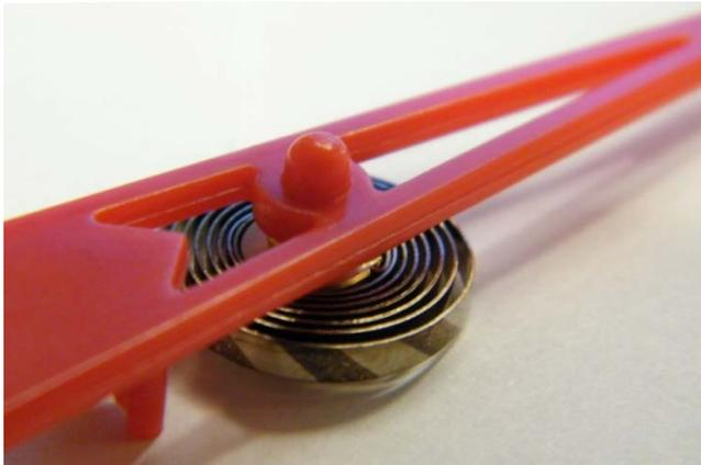
Figure 2 Bimetallic strips are often used in thermostats and thermometers. Here, we use one to create a dynamic tag that indicates temperature.
