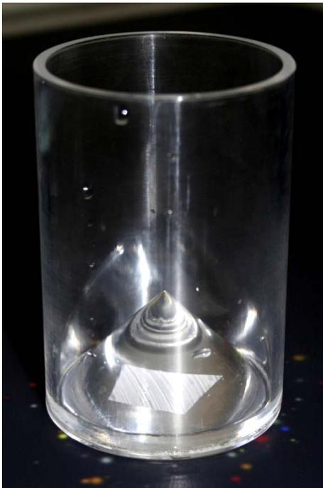
Figure 9. A SurfaceWare glass with a single large reflector is shown. This allows for an analog measurement of fluid level once the drink level has progressed down to the tip.
