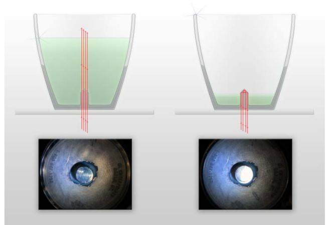
Figure 7. The test cup is illuminated from underneath with a flashlight. It is easy to distinguish the fluid level by the reflection.
