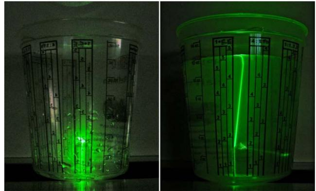
Figure 6. The test cup is shown with a laser pointer shining up through the plastic rod. In the left picture, the cup is empty, so the tip reflects. In the right picture, the tip is submerged, and the beam escapes up through the fluid.
