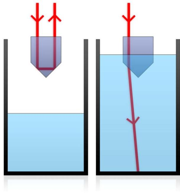
Figure 3. Gems Sensors optical liquid level sensors reflect light when the tip is in air, but do not when submerged.
