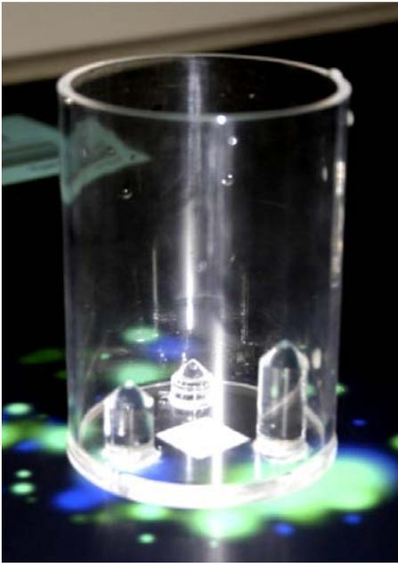
Figure 8. This SurfaceWare glass has three reflectors to allow a more detailed measure of drink progress.
