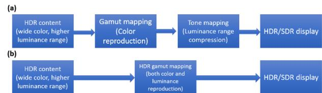
**Figure 2.** (a) Display pipeline for HDR contents on contemporary TV and (b) the proposed HDR gamut mapping algorithm.
